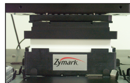
Figure 3. FiltrEX™ 384 well Filter Plate in the Positive Pressure Filtration Unit
