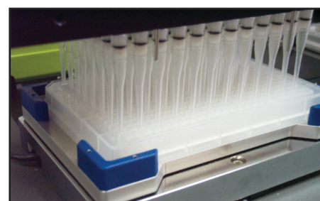
Figure 2 - 384 well microplate on the deck mounted shaker.
