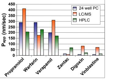
**Figure 2: Drug Transport analysis of known compounds.** Several compounds of known permeability were tested for transport in Caco-2 cultures. After incubation for transport, samples were collected and analyzed via either HPLC or LC/MS. In these studies, HTS Transwell®-96 permeable supports with the polycarbonate membrane were used. Apparent permeability shown is for the A>B direction. Each compound was tested in at least 6 wells in at least 3 independent experiments.
