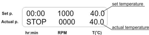
Fig.4 Control panel in operation mode
