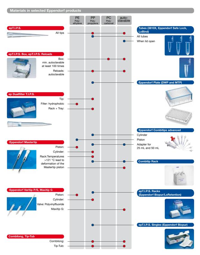
Eppendorf epT.I.P.S., Tubes and Combitips advanced are also available in Eppendorf Biopur quality, i.e. sterile, free of RNase, DNase and PCR inhibitor, human and bacterial DNA, Pyrogen and ATP. epT.I.P.S., Tubes and Combitips advanced are also available in PCR clean quality, i.e. free of human DNA, DNase, RNase and PCR inhibitor.
