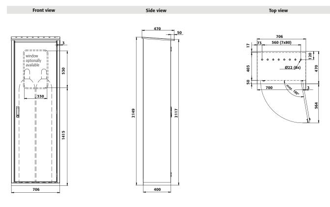
Diagram shows left-hinged door. Dimensions are identical for a right-hinged fitting.
