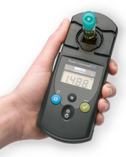
The Pocket Colorimeter II has already proven its worth, but now it can serve additional application areas: These single parameter meters can now be used for key parameters to evaluate **LCK cuvette tests** in addition to traditional Hach methods. This dual functionality enables you to make the most of two key benefits: cost-effective meters combined with reagents for various quality standards. The result? Outstanding portable water analysis.
