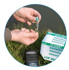
Out in the field: Samples are added directly for the pre-configured LCK cuvette test. The cuvette is ready for use after a short development time.
