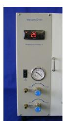
A vacuum gauge is fitted showing vacuum pulled, from 0 to 1000 mbar.
