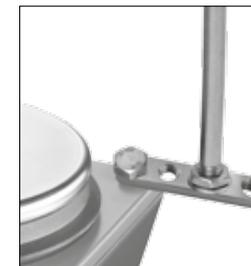
Note: When using bath attachments with a diameter over 180 mm, please use support rod in conjunction with an extension. (See "**Accessories**")
