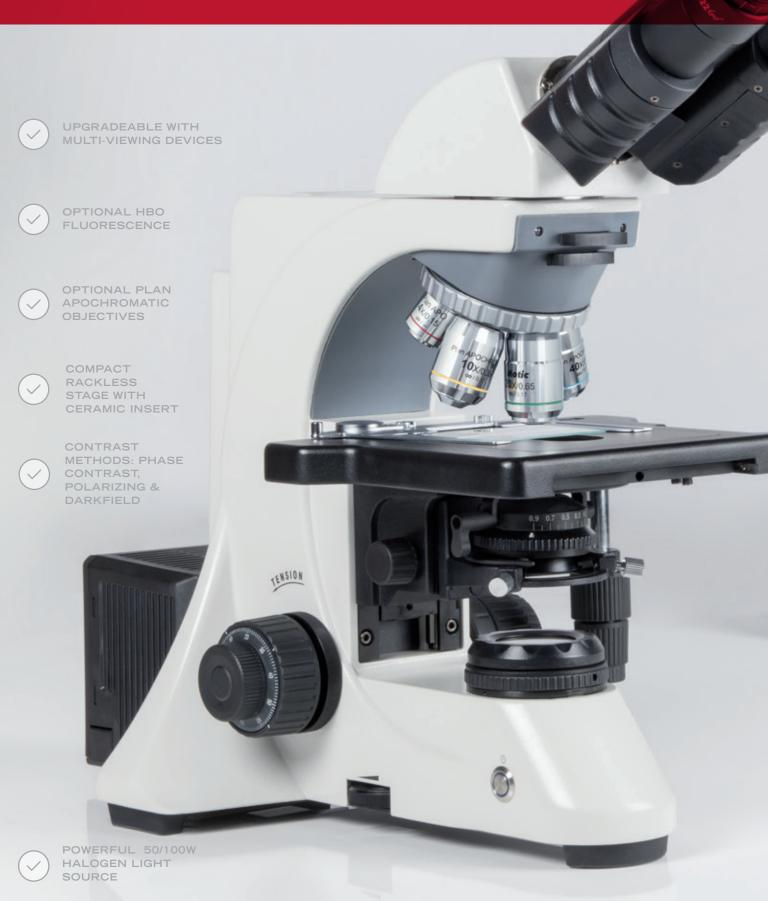
(positive & negative), Polarization contrast with compensator I. Order RED, Darkfield and Multi-Viewing devices. HBO Fluorescence can easily be added. The rackless stage with a ceramic stage insert allows a safe positioning and fast throughput of slides for a long lifetime. The BA410E is a flexible microscope platform with multiple options to configure a workstation which perfectly suits individual demands.
