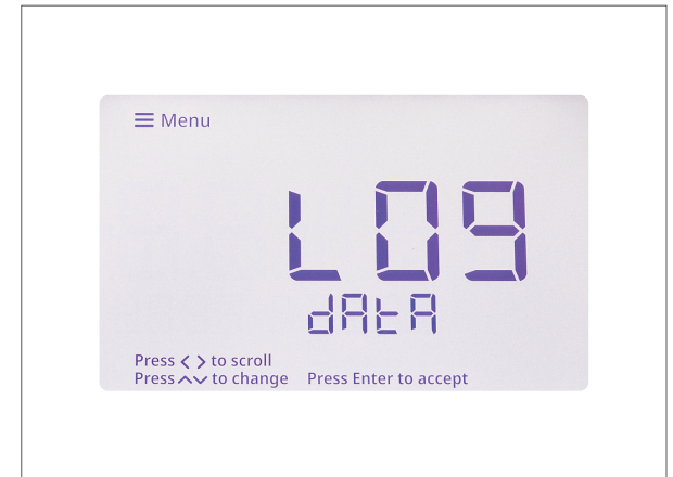
Critical data is automatically saved to the meter's 500-point data log.
