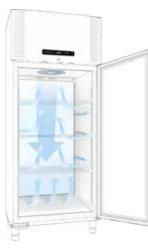
**Optimised air flow** The unique Gram BioLine air distribution system makes sure that the temperature is consistent everywhere in the cabinet and that the time taken to return to the programmed temperature after a door has been opened, is very short.
