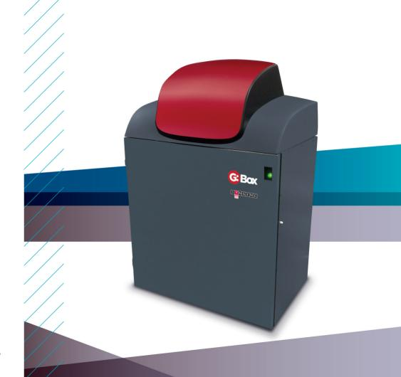
The **InGenius 3** gel documentation and analysis system is compact and easy to use. The system has a small footprint darkroom featuring a CCD camera, manual zoom lens and a filter drawer. Internal lighting comes from an optional UV or blue light transilluminator (for safe dyes), both of which can slide in and out of the darkroom for ease of access.
