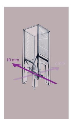
The patented\* Eppendorf UVette is a fully UV-transparent, single use cuvette made of clear plastic, with a light transmission of 220 nm to 1,600 nm. The unique design allows you to conduct flexible measurements with two different light paths (10 mm and 2 mm).
