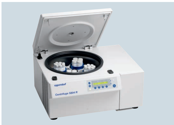
Centrifuge 5804 R with rotor S-4-72 (4 x 250 mL)
