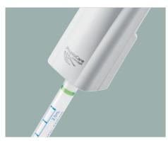
**Multipette connection** Automatic Combitip recognition and volume calculation
