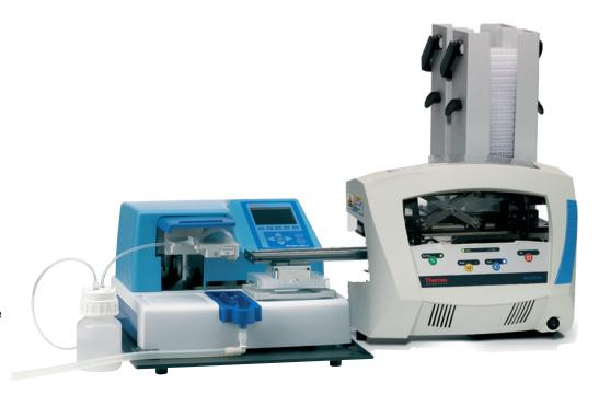
The RapidStak stacker with the Multidrop Combi nL dispenser creates a complete benchtop solution for automated low-volume reagent dispensing.
