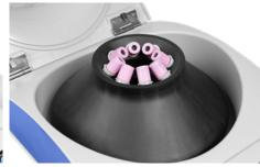
Rotor fits a multitude of tube sizes with the included tube adapters and spacers
