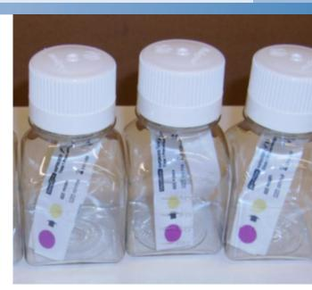
Figure 1. VHP process indicator strips inside 125 mL media bottles.
