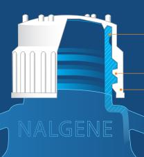
**Seal Ring** is molded inside the closure. It fits tightly against the beveled inner edge (chamfer) of the bottle neck. For dis-similar materials (e.g., HDPE carboy with PP closure) no gasket is required. For PP-to-PP sealing a gasket is added for extra security of the seal.
