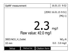
In addition to the measured value, an evaluation number for the measurement quality (MQ) is shown on the display and stored with the measured value.
