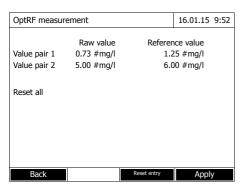
With a 2-point calibration, by selecting the corresponding value pairs the characteristic curve can be optimized by adjusting the slope and / or the offset.
