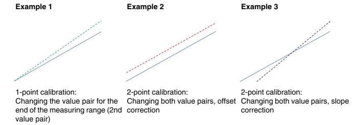
If the deviations predominantly occur in the lower **or** upper measuring range, a 1-point calibration in the relevant range of the deviation is normally sufficient. If, however, the differences are in the whole measuring range or there is an offset, a 2-point calibration has to be carried out. An offset deviation can be identified by a constant difference between raw value and reference value.
