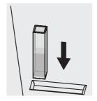
Pipette the sample into a 10 mm quartz photometer cell cell.
