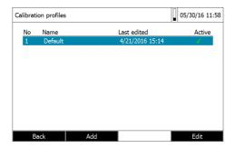
4 Select [Add] with the function key F2. Enter and confirm a name for the new calibration profile.
