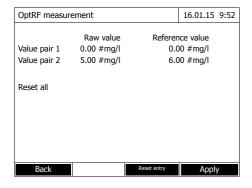
For a 1-point calibration, a suitable value pair from the beginning or end of the measuring range is entered in the input fields. The other value pair remains unchanged. In this example, the upper value pair (value pair 2) is entered. Thus only the slope but not the offset of the characteristic curve is changed.
