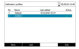
**6** Create further calibration profiles with [Add] or return to measuring or the user calibration with [Back].
