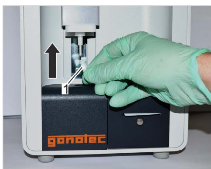
Fig. 70: Position measurement vessel
