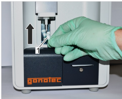
Fig. 94: Position measurement vessel
