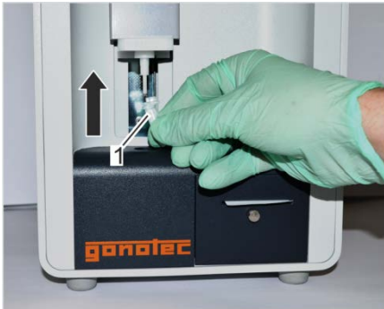
Fig. 52: Position measurement vessel
