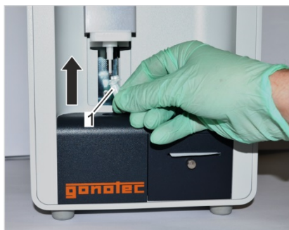
Fig. 19: Position measurement vessel
