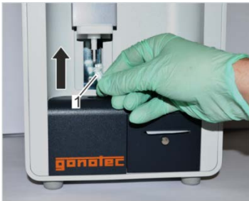
Fig. 82: Position measurement vessel
