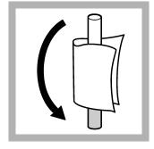
**8.** Thoroughly clean the outside of the indicator cuvette and evaluate. **Do not invert.**
