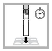
Heat in the thermostat (blue indicator cuvette upwards).
