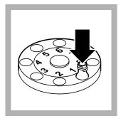
2. Insert the open digestion cuvette in the TOC-X5 shaker, pushing it down as far as it will go. Position the fan cover over the cuvette. Switch on the instrument. After 5 minutes an acoustic signal is emitted.
