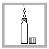
**1.** Pipet **0.1 mL sample** into the digestion cuvette.
