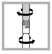
**7.** Tighten the cuvette combination again.
