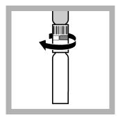
**4. Immediately** close the digestion cuvette tightly with the prepared indicator cuvette. Hold cuvette combination vertically.
