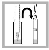
Slowly pipet into the Cuvette Test: 0.5 mL of digested sample.
