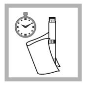
4. After 5 minutes, thoroughly clean the outside of the cuvette and evaluate. Any air bubbles sticking to the wall of the cuvette can be removed by giving the cuvette a short sharp shake or by tapping the cuvette gently against a surface.
