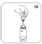
Hold cuvettes vertically and Add 10 drops KS61 (Ferro-
