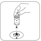
Remove the vial from the sample chamber.
