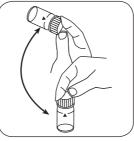
Dissolve tablet(s) by inverting.
