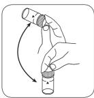
Dissolve tablet(s) by inverting.
