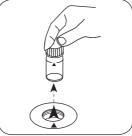
Remove the vial from the sample chamber.
