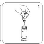
Place 1 drops Vario **ALUMINIUM ECR Masking** Reagent in the blank.
