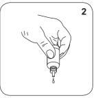
Add 2 drops KS135 (Phenolphthalein Substitute Indikator).
