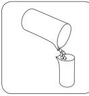
Fill a suitable digestion vessel with 50 ml homoge- sulfuric acid). nised sample.
