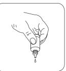
Add KS 144 (Calcium Hardness Buffer) drop by drop to the same sample until colouration turns from light pink to red. (Note: make sure to swirl the vial after adding each drop!)
