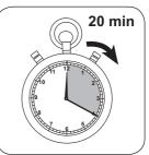
Boil the sample for 20 minutes. A sample volume of about 25 ml should be retained; If necessary, fill with deionised water.
