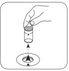
Remove the vial from the sample chamber.
