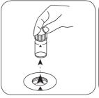
Remove the vial from the sample chamber.
