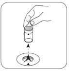
Remove the vial from the sample chamber.
