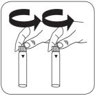
Prepare two digestion vials Open the vial. TN Hydroxide HR . Mark one as a blank.
