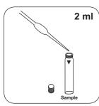
Fill sample vial with 2 ml prepared, digested sample.
