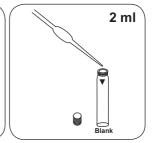
Place 2 ml of digested, pre-prepared zero sample in the blank.
