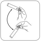
Allow vial(s) to cool to 60 °C. Invert several times to mix the contents.
