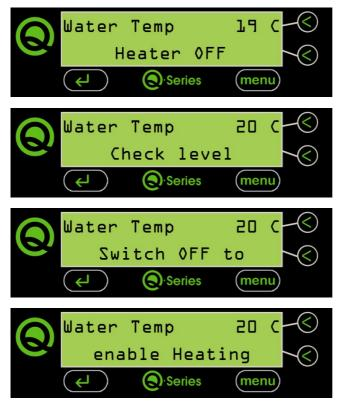
To continue using your SLS Lab Pro ultrasonic bath, refill with liquid up to the level sensor, switch the unit off and on again.
