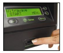
The memory card can be connected to a PC, using this memory to USB card reader to give a permanent electronic record of the cleaning parameters of the cycle.
