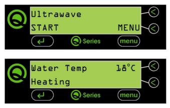
When the water temperature is at or above the temperature set, the message "Temp OK" will display.
