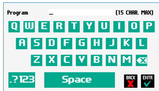
New Program Name Entry screen showing letter keys. To view numbers/symbols, choose the use button ?123 in the lower left corner
