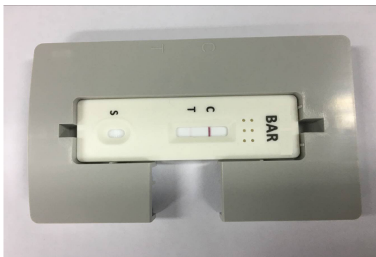
Fig.17 The placement of test cassette in the cartridge
