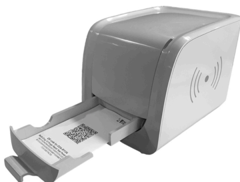
Fig.11 Place QR code Card in the cartridge tray and then insert the tray into the Reading Area
