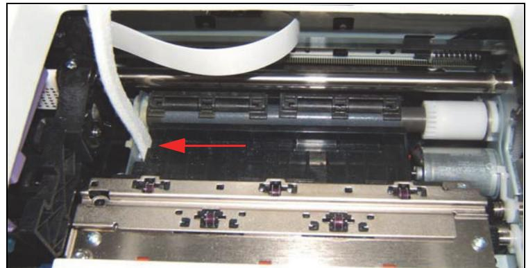
11. Fold felt strip down into trough so small tabs fit into notches on felt.
