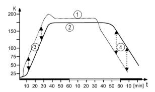
Schematic temperature sequence internal/external
