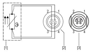
Connection of a external Pt100 temperature sensor
