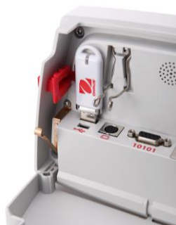
Interface connections inside of the Terminal.
