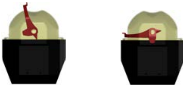
Figure 2-20: Bucket with open lid (left) and closed lid (right)
