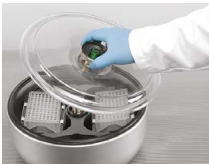
Figure 2-8: Put on/off the rotor lid
