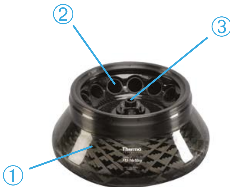
① Rotor body; ② Cavity; ③ Rotor lid mounting
