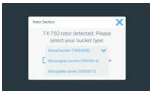
Figure 2-17: Rotor Detection: Choosing a Bucket Type for a TX-750 Rotor
