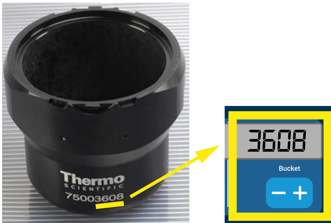
Figure 2-18: Setting the Correct Bucket Code
