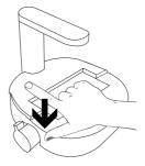
**Figure 15.** Carefully press the adapter plate downwards.
