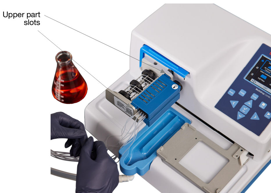
Figure 4–16. Lower and upper parts of the dispensing cassette inserted evenly into their slots
