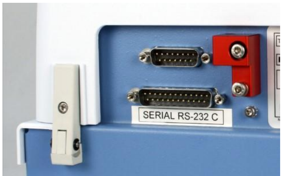
Figure 3–7. Transport lock storage
