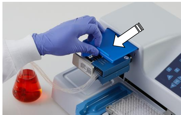
Figure 6-58. Pulling the rotor cover over the rotor
