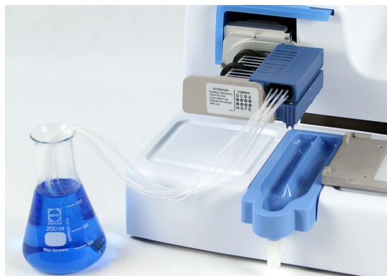
Figure 4–20. Cassette with the tip and tubing weight protections removed, and the tubing weight in the reagent vessel
