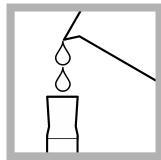
2. Prepare the sample: Fill a mixing cylinder to the 20mL line with sample.
