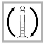
mixing cylinder. Invert the mixing cylinder several times to fully dissolve the powder. Undissolved reagent causes
