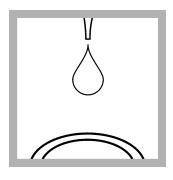
**9.** Add 1 drop of ECR Masking Reagent Solution into a clean square sample cell.
