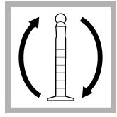
7. Put the stopper on the mixing cylinder. Invert the mixing cylinder several times to mix.
