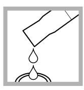
8. Pour 10 mL of the solution from the mixing cylinder into the sample cell.
