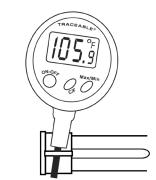
Insert the probe into the "loop" on the cover. It makes a perfect holder.
