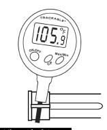
Insert the probe into the "loop" on the cover. It makes a perfect holder.
