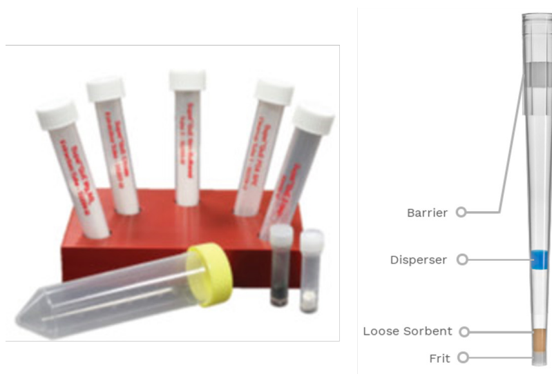
Figure 23. Dispersive Solid Phase Extraction (dSPE) Formats. Shown on the left are traditional Quechers tubes whose typical method is outlined above. On the right, a newer format shown is dispersive SPE tips that is comprised of loose sorbent within a micropipette tip, allowing the extraction to be performed entirely within the tip in a method that entails simple pipetting steps.
