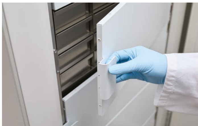
Figure 6: Every door opening of an ULT freezer results in a warm-up of the inner compartment which requires a fast pull-down back to the setpoint
