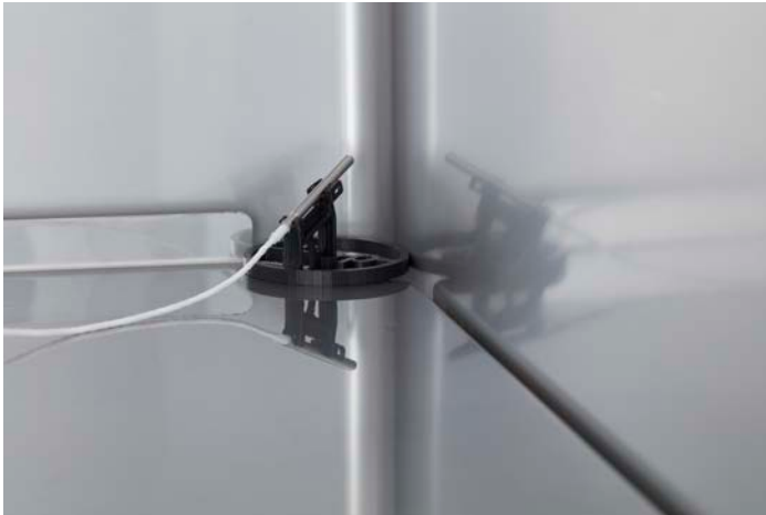
Figure 2: Temperature probe positioned within freezer cabinet
